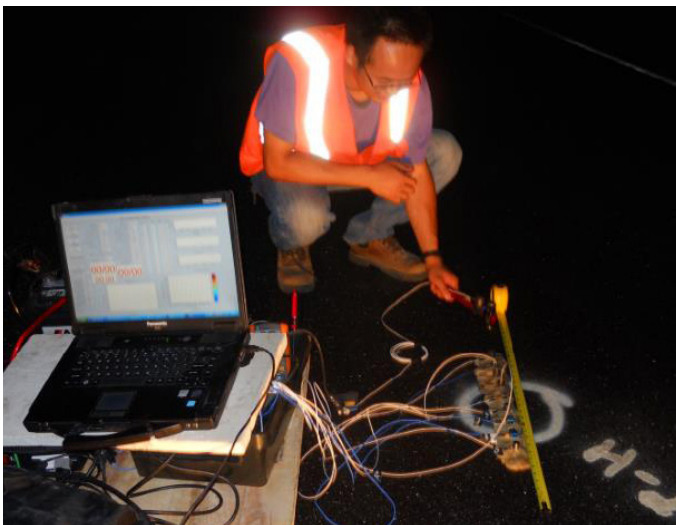
Figure 1. Surface wave testing on US 6
