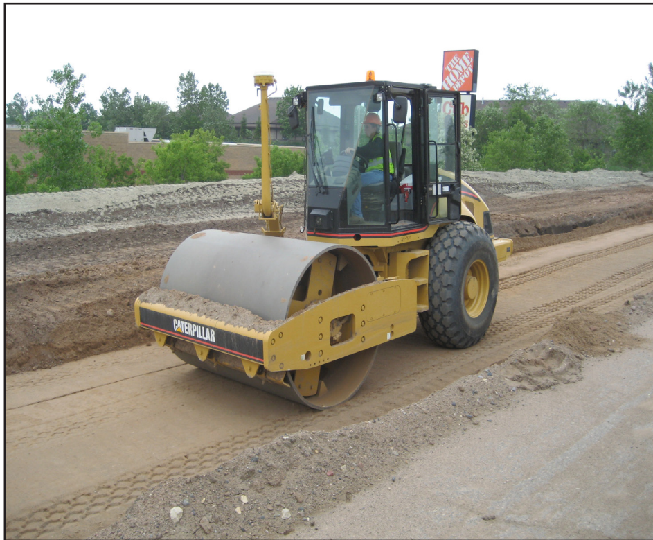
Figure 1. Caterpillar CS563 padfoot roller with CMV measurement system on TH 36 project (White et al. 2009)
