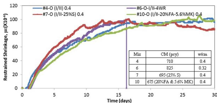
**Group 2 restrained shrinkage:** While showing lower shrinkage values than Mix 7, all three Mix 6 ring specimens cracked, at 16, 16.5, and 18 days, and two of three Mix 4 specimens cracked, at 13 and 18 days
