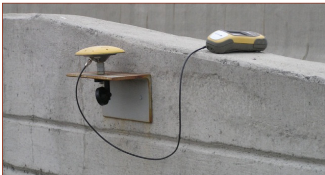
Total station prism and GPS antenna on Bridge 0309 at north abutment
