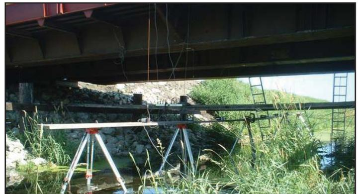
*Deflection instrumentation installed below RRFC bridge*
