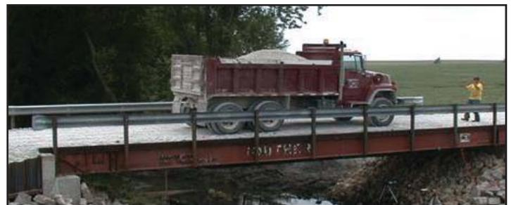
*Test truck driving across single span RRFC bridge*
