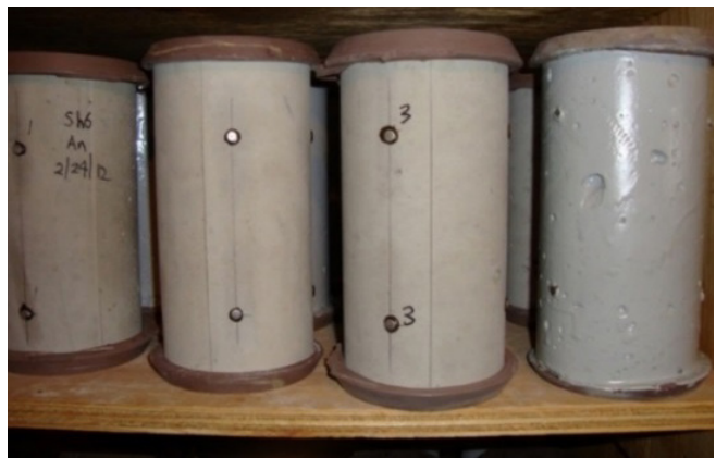
Loaded specimens for creep tests in environmentally controlled chamber (top) and shrinkage test specimens in environmentally controlled chamber (bottom)
