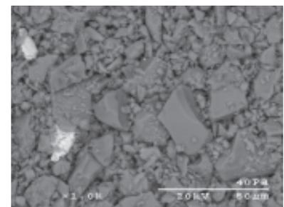
*Slag viewed through scanning electron microscope*
