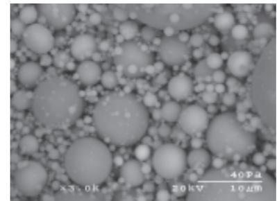
*Fly ash viewed through scanning electron microscope*
