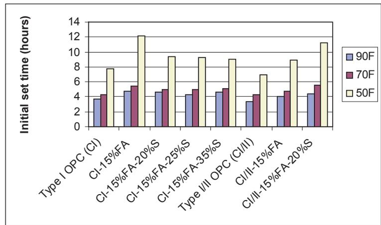
*Initial set times of concrete made with Type I and Type I/II OPC and various amounts of fly ash and slag at 90°F, 70°F, and 50°F*
