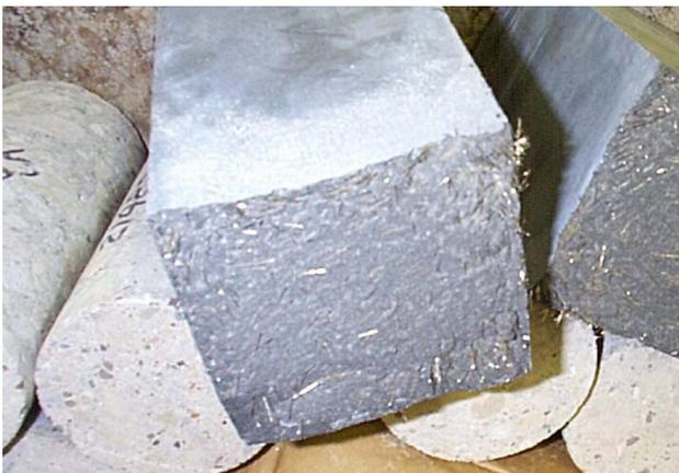
*UHPC samples on top of conventional concrete samples*
