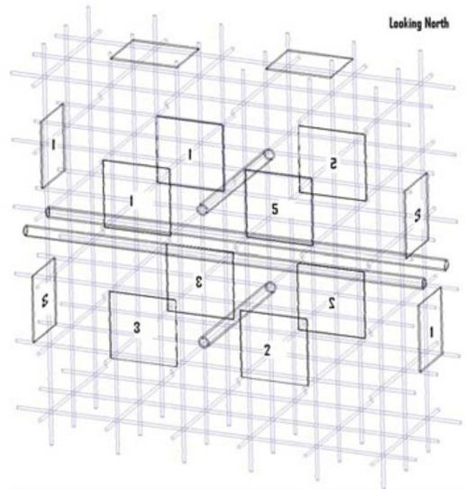
*Drawing showing the interior of the Midway block and the locations of the subsurface defects in relation to the block.*
