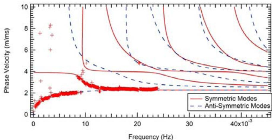
*An example of the dispersion curves generated from both the theoretical (represented by the solid thin red and dotted blue lines) and experimental studies.*
