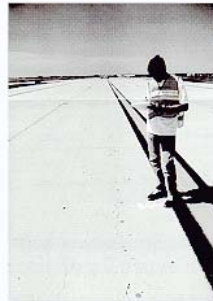
An engineer from Applied Pavement Technology records data during a pavement evaluation survey.
